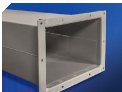
12-gauge (2.75 mm) fixture welded trunking is standard on all YORK powder-coated and galvanized bucket elevators, with 10-gauge (3.41 mm) trunking available on request.
