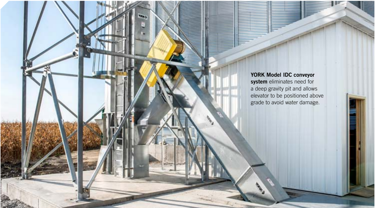
Direct drive motorized torque arm (available on request) eliminates need for belt drive and belt guard. Unit is self-contained.
