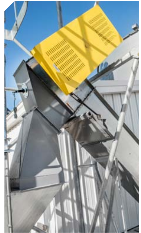
All Dodge speed reducers come furnished with a drive guard that meets OSHA standards .
