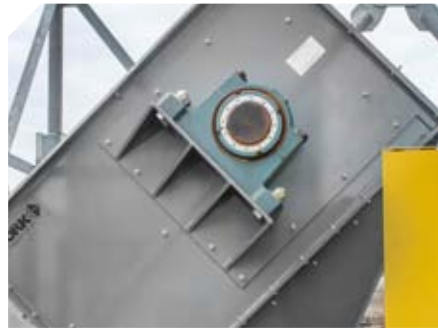
Heavy-duty gusset channels keep head and bearings rigid and stabilized during operation.
