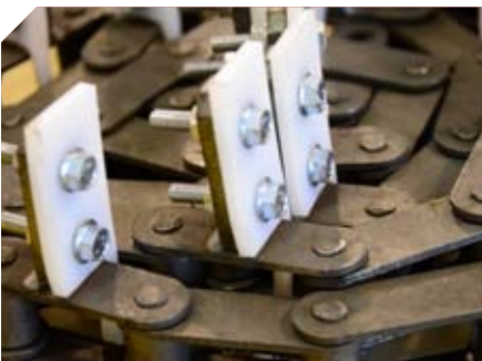
Conveyor chain and paddles ship pre-assembled for more efficient, time-saving installation in the field.
