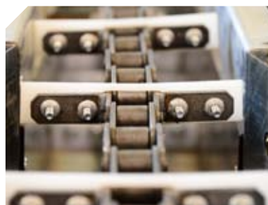
Pre-assembled conveyor chain and paddles help reduce cost and accelerate field installation.
