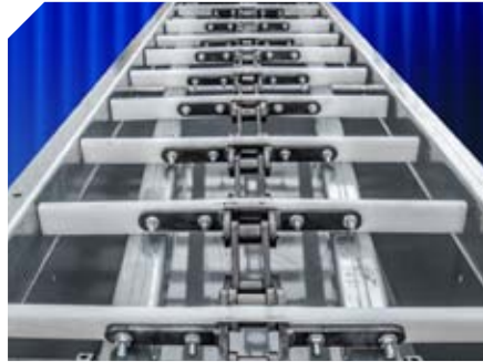
Double-flighted chain standard on all under floor conveyors.
