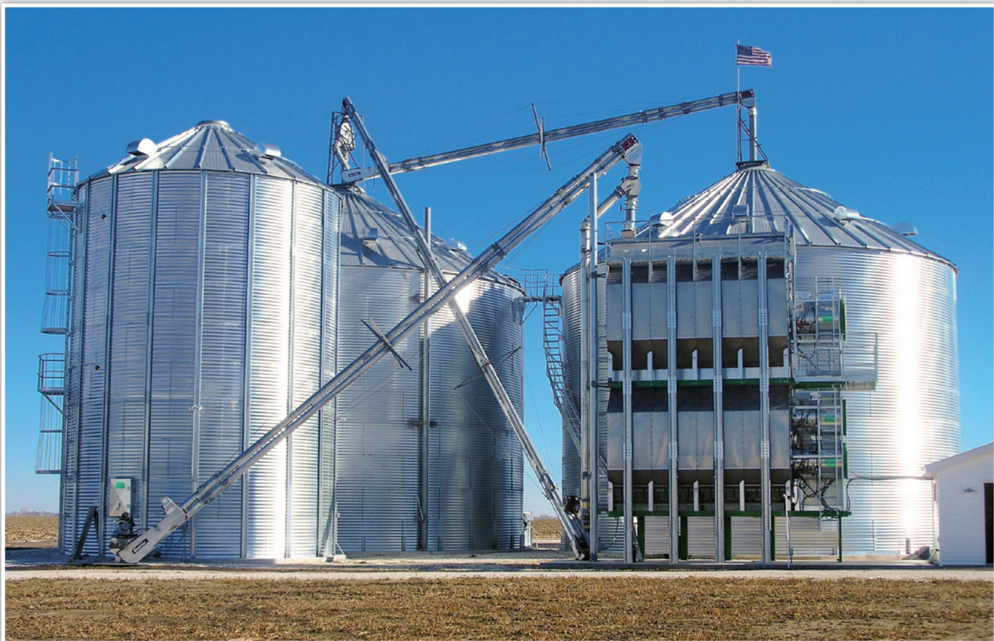
Stationary Double Run filling a dryer and unloading dryer to multiple bins. Eclipse Towers and Hutchinson Truss Kits are now available.
