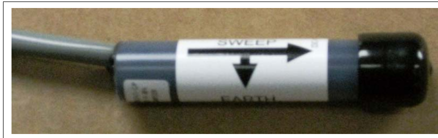
Figure 3 Accelerometer Assembly Installation
