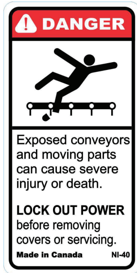
Figure 7 Moving Chain Hazard NI-40
